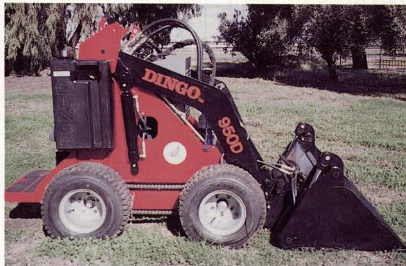
DINGO 950 PETROL OR DIESEL 20HP TWIN HYDRAULIC PUMPS
